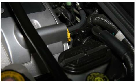
tends to ride against the fuel rail cover. Since one end of this line is fixed to the firewall and the other to the fuel rail, this line is constantly rubbing against the edge of the fuel rail cover as the engine shifts left and right during normal driving. Obviously, more aggressive driving causes even more relative motion and consequently more rubbing.
